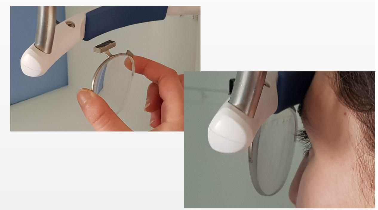
A set a large field lenses (55 mm in diameter) prevents errors resulting from the lens rim or lens misalignment in visual field perimetry and multifocal ERG exams.
