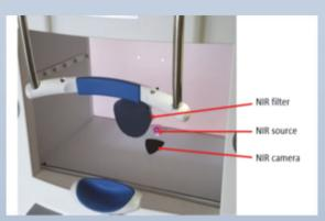
The high-resolution video sensor combined with advanced image processing measures the position of a reflective dot to determine the movements of the head. The positions of the pupils in relation to this patch are used to determine the movements of the eyes.
