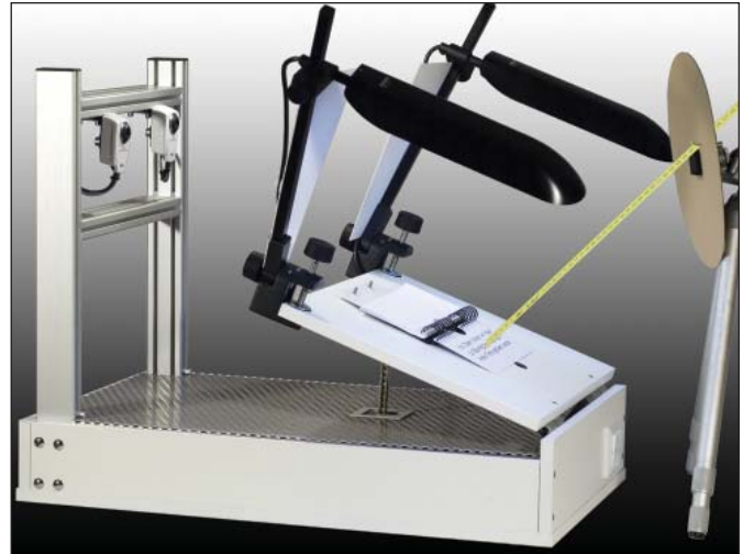
Figure 1. Side view of the Salzburg Reading Desk (SRD). Camera tripod with cardboard and green color-coding dot simulating a test situation in front of the SRD. Yellow meter ruler for reference distance measurement in front of the SRD.
