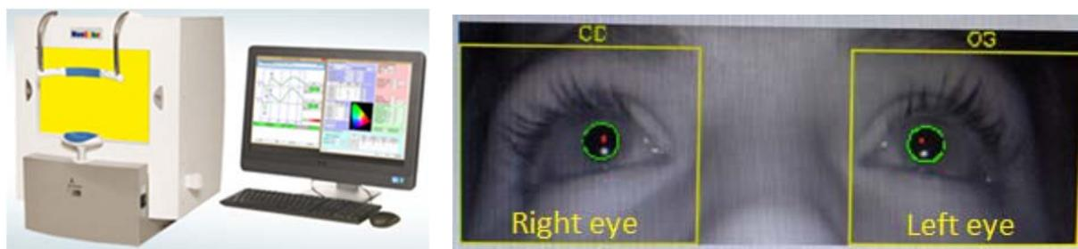
**Figure 1 – MonColor chromatic pupillometry device (left), view of the participant's eyes with the infrared cameras (right)**
