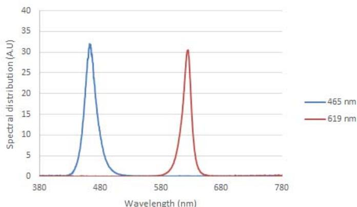
**Figure 2 – Blue and red LED spectra centred at 465 nm and 619 nm respectively**
