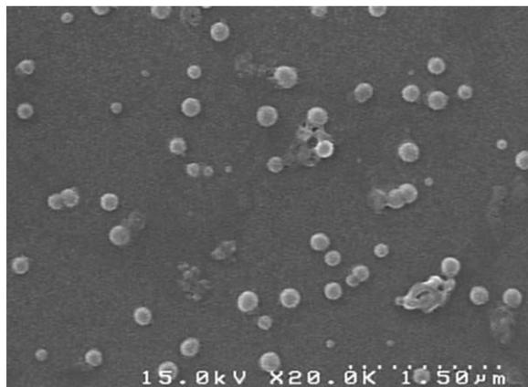
**FIGURE 1.** Scanning electron microscopy image of prepared nanoparticles containing bevacizumab.
