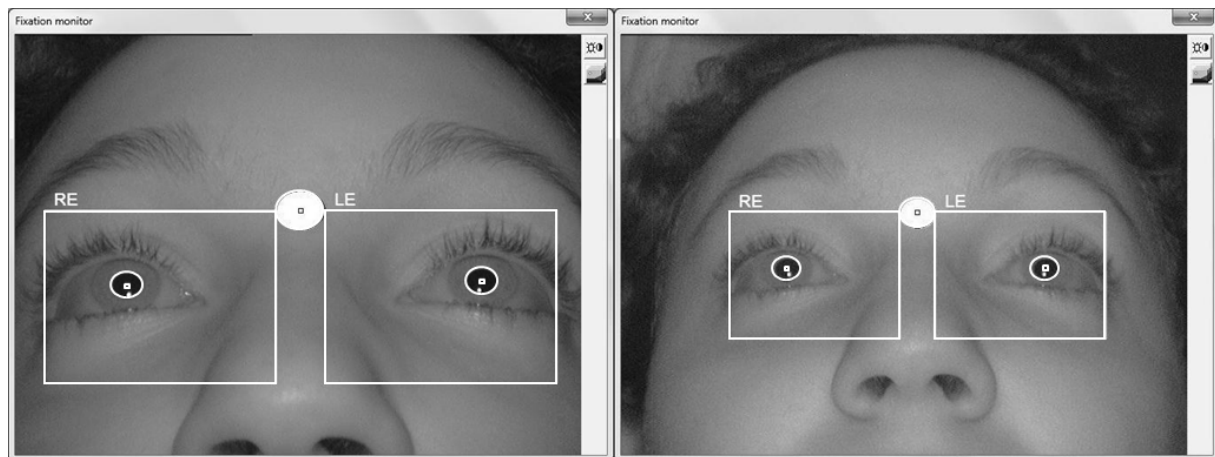
Figure 2 detection of the reflective dot and the two eye pupils as a function of the distance to the camera: (a) at 33cm, (b) at 45cm
